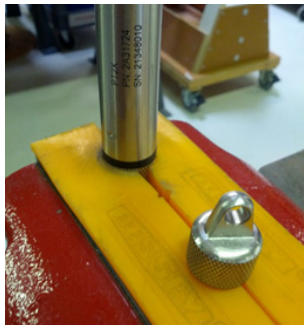
Cableless Sensor—gripping on knurled area
