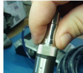
Properly completed—black ring uncompressed
