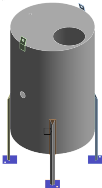
Figure 5 Fixed Support boundary condition
